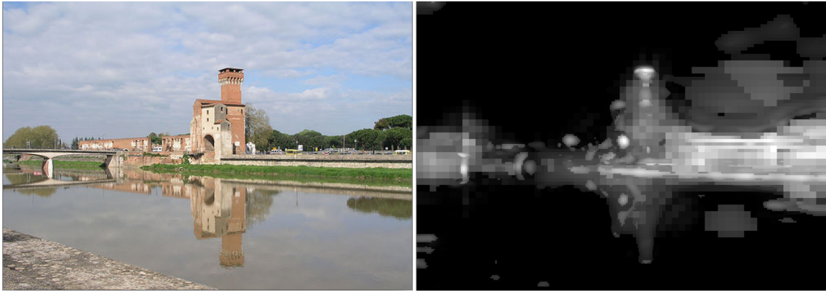
Figure 1: Example of the application of the visual attention model. Left: original image; Right: saliency map computed by the model: the brighter the pixel the more salient the area surrounding it is.
