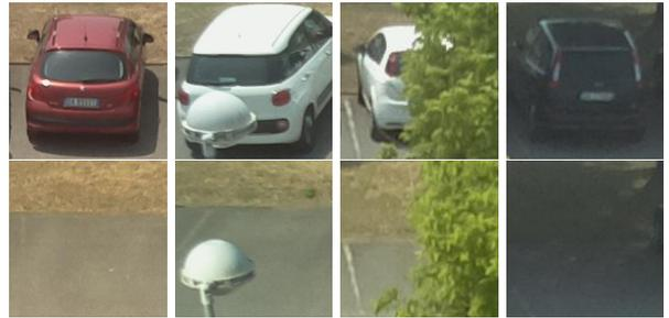
FIGURE 3: TRAINING SET PATCHES SEGMENTED FROM THE CAMERA VIEW. IMAGES SHOW FOUR PARKING SPACES IN BOTH STATUS: BUSY (FIRST ROW) AND FREE (SECOND ROW). THEY ALSO PRESENT SOME OCCLUSION AND SHADOW SITUATIONS THAT WE FACED.
