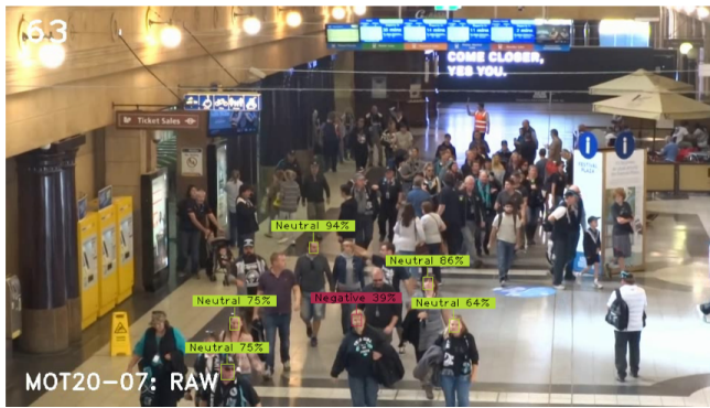
Figure 2. Example of the output of our Facial Expression Recognition system. We recognize human facial expressions by automatically analyzing images.
